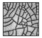
pattern of "crazing" is different from a crack in the aspect that it cannot be felt on the surface, unless using a fingernail; however it does become more visually apparent when the surface is dusty or magnified. While this "crazing" may appear as imperfections, crazing does not affect the performance of life span of your ceramic BBQ; therefore it can't be claimed as a warranty issue. The process of crazing effectively increases the toughness of the unit.
