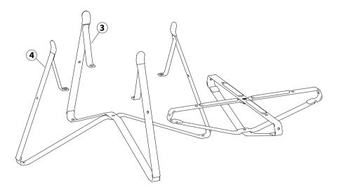
**STEP 2:** Take frame part 3 and frame part 4 and form another 90 degree cross by alligning the center hole. Slide in the cross from step 1 from the side till both center holes allign.
