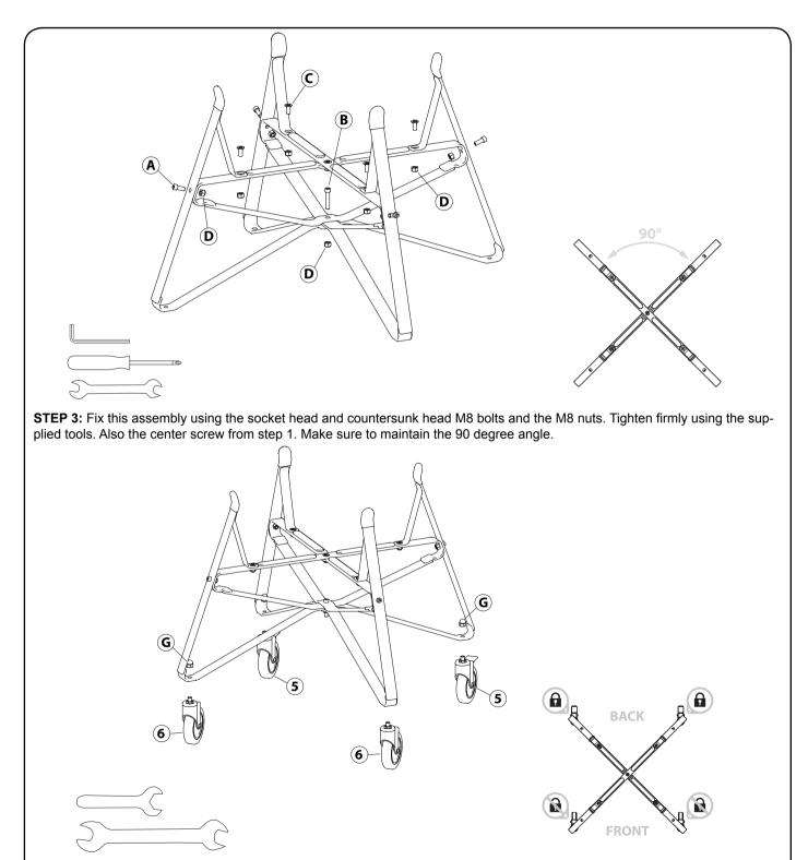
**STEP 4:** Insert the wheels (item 5 & item 6) in the bottom holes. Please follow the diagram below to know where the castor wheels with brake need to be installed. Fix the wheels to the frame with M10 domed nuts (G) using the supplied tools.
