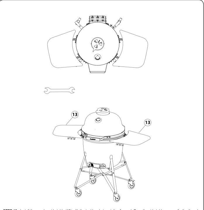
**STEP 10:** Install the wooden side table (13) with the tool brackets pointing forward. Once the side tables are perfectly aligned in the brackets, fix the domed nuts firmly using the supplied wrench. Side tables can be folded down by slightly lifting them up and sliding them outward. For storage or cleaning, they can also be removed if needed by lifting them out of the slots, through the opening.
