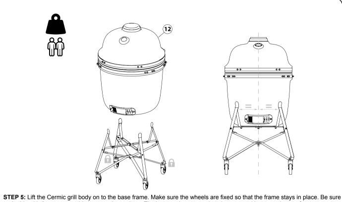
**STEP 5:** Lift the Cermic grill body on to the base frame. Make sure the wheels are fixed so that the frame stays in place. Be sure to do this with 2 persons as this is a very heavy item. The bottom air vent needs to be centered between the two front support brackets.
