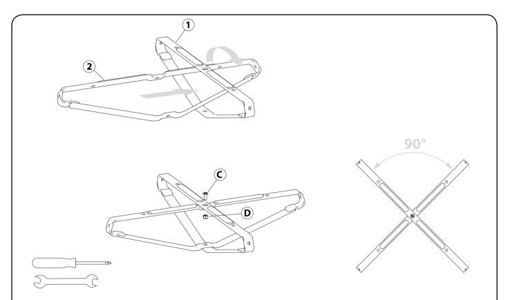
**STEP 1:** To assemble the base frame, start by inserting frame part 2 inside frame part 1 to form a cross. Fix the cross in a 90 degree angle by using a countersunk M8 bolt (C) with a M8 nut (D). Handtighten till after the complete frame is assembled.
