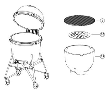
**STEP 6:** Open the lid of the ceramic grill to insert the fire box (11), fire grate (10) and the grill grate (9) in the order indicated on the diagram.
