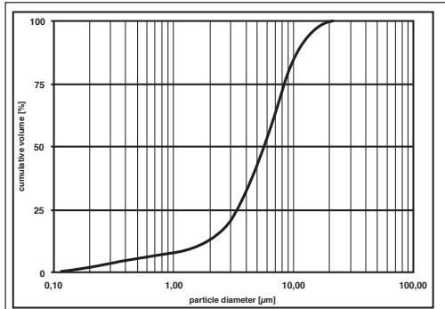
All measurements were obtained with a sodium chloride solution using a laser diffraction method. This diagram may not be applicable for suspensions or highly viscous medicines. More information can be obtained from the relevant medicine manufacturer.
