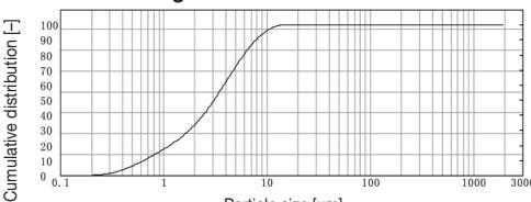
All measurements were obtained with a sodium chloride solution using a laser diffraction method.
