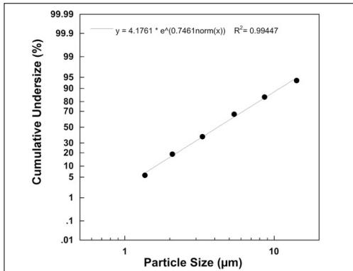
Measurements were performed using a sodium fluoride solution with a "Next Generation Impactor" (NGI).
