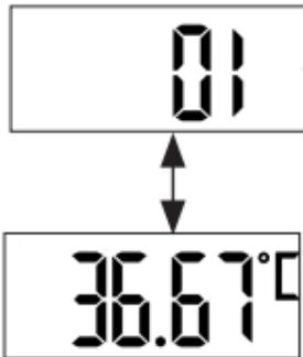
3. In order to navigate between the saved measurements, repeatedly press the on/off button briefly. In order to leave the memory menu again and switch off the device, press and hold the On/Off button for three seconds.
