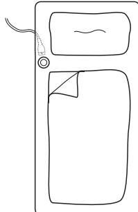
Make sure that the electric underblanket is always smoothed out flat and does not crumple or form folds during use. When making the bed, check the position of the electric underblanket – it must only be switched on when it is flat and smoothed out. We recommend switching on the electric underblanket approx. 30 minutes before going to bed and covering it with the duvet in order to prevent heat loss.
