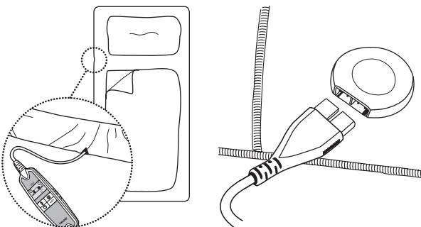
Then pull the side section over the sides of your mattress like a fitted sheet. The electric underblanket is designed to fit 90 x 200 cm as well as 100 x 200 cm mattresses. If the cable length is insufficient, you can order a longer power supply cord with the material number 108.424 from our specified Customer Service. Then fit your fitted sheet as usual with the electric underblanket positioned between your mattress and the fitted sheet.
